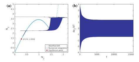
Fig. 7.3 a SIM of the system with the numerical integration of the scaled Sys. (7.2) under small forced oscillations with f = 0.3 and the detuning parameter  $\sigma = 0$ . b Time histories of the velocity  $dy_1/dT$
