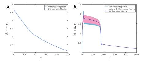
**Fig. 7.1** Time histories of  $|dy_1/dT + i\omega y_1| = N_1$  and  $|dy_2/dT + i\omega y_2|$  obtained by the direct integration of Sys. (7.2) under free oscillations; i.e. f = 0
