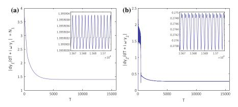
**Fig. 7.4** Time histories of both amplitudes  $|dy_1/dT + i\omega y_1| = N_1$  and  $|dy_2/dT + i\omega y_2|$  obtained by the direct integration of Sys. (7.2) under small forced oscillations with f = 0.3 and the detuning parameter  $\sigma = 0$
