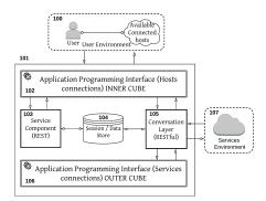
Fig. 2: CUBE works with multiple devices and services
