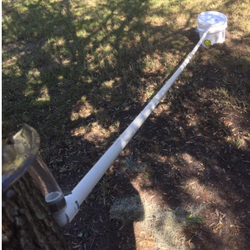
Figure 14.4. Manipulation experiments are needed to explicitly address research questions at the intersection of precipitation partitioning processes and the plant microbiome. This photo is an example stemflow collar outfitted to redirect flow to an area typically receiving throughfall (credit: John T. Van Stan, II). A video of SF redirection from this system is provided in the supplemental materials [ https://youtu.be/AKhRV6Q7hGM ].
