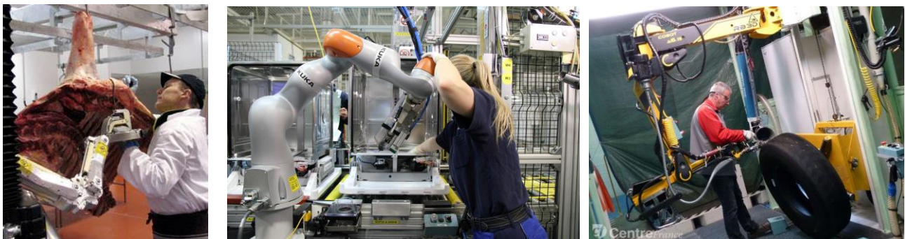
Figure 1: Examples of collaborative robots for industrial applications. Left: HookAssist (Kinea Design) for beef boning. Center: Lightweight robot (KUKA). Right: Cobot 7A.15 (RB3D) for tire retreading.
