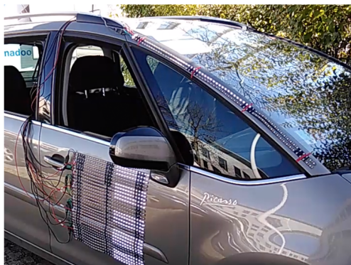
Figure 1: 3D simulation, design and prototype of our external Human-Machine Interface for autonomous car.
