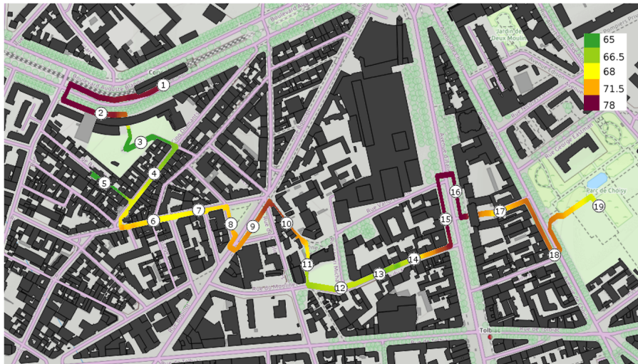
Figure 1: Noise map of the path and 19 locations of the soundwalks presented in [11]. Sound levels (Leq in dB SPL) were measured at each of the 19 locations and interpolated to obtain a sound level estimations along the path.
