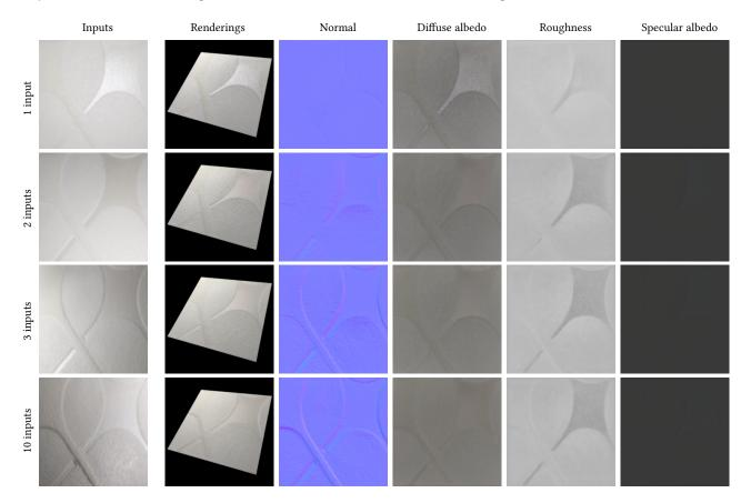
Figure 3: Evaluation on a measured BTF. Three images are enough to capture most of normal and roughness maps. Adding images further improves the result by removing lighting residual from the diffuse albedo, and adding subtle details to the normal and specular maps.
