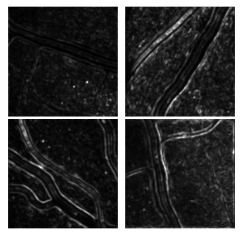
Figure 7: Trace images corresponding to the input of Figure 5, and the tensor field  $T_{\sigma}$  with  $\sigma = 3$ . They can be seen as smoothed version of the square norm of the  $\nabla f$ .
