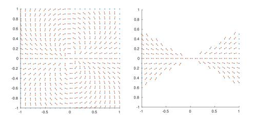
Figure 9: Left: a set of elements  $(p, \vec{v})$  co-circular to the central element  $(p_0, \vec{v_0})$  where  $p_0$  is the origin and  $v_0 = (1,0)^T$ ; Right: the elements form the left hand image that comply with the additional constraint that the (smaller) angle between the directions defined by  $\vec{p_0p}$  and  $\vec{v}$  is smaller than  $\frac{\pi}{6}$ .
