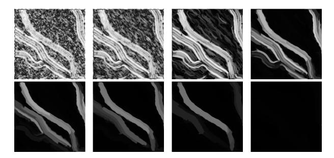
Figure 11: Example of openings  $\gamma_W^{(p)}$  on an anisotropy image, in the case of a binary and symmetric matrix W, computed as explained in Section 4.1.1. From left to right, top to bottom: p = 0 (original anisotropy image), p = 1, 5, 15, 20, 30, 40, 60. The parameters used here are k = 7 (spatial window),  $\alpha = \frac{\pi}{20}$  (cocircularity precision) and  $\beta = \frac{\pi}{6}$  (conic constraint).
