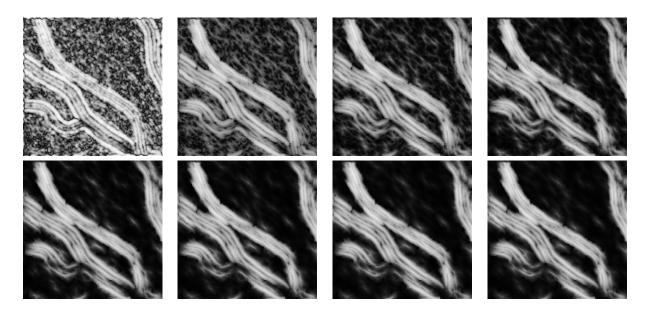
Figure 13: Sequence of anisotropy images defined as in Section 4.2.3. In this example p = 4, and from left to right, top to bottom: n = 0 (original anisotropy image), n = 1, 2, 3, 5, 7, 10, 13. After n = 13, no significant change occurs.
