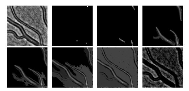
Figure 10: Illustration of the geodesic reconstruction by dilation. From left to right, top to bottom: mask image *I* (in this case, the original image); marker image *R* (defined manually);  $I_5$ ,  $I_{25}$ ,  $I_{35}$ ,  $I_{50}$ , final reconstruction  $\tilde{I} = I_{178}$ ; residual image  $I - \tilde{I}$ .
