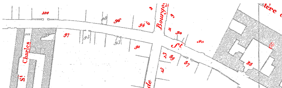
Figure 1. In this example, handwritten text is automatically detected and extracted (red) from a historical map using various image processing methods. Note that some building numbers are not extracted.
