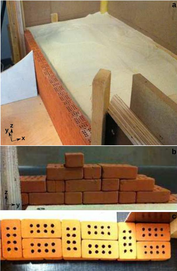
Figure 1: a) Box for the experimental set-up. Focus on the arrangement of bricks within the wall; b) Frontal plane view; c) Horizontal plane view.
