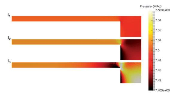
Figure 13. Pressure distribution in the real capsule for different times. The sample is not represented for the sake of simplicity.
