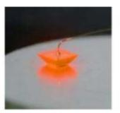
The LED die consists of epitactical layers of doped semiconductors (III-V): one n-conductive layer with a surplus of electrons and a p-conductive layer with a lack of electrons (or surplus of "positive" holes) and the depletion layer in between. When a voltage is applied, the electrons in the n-layer have enough energy to cross the depletion layer. They recombine with the holes in the p-layer and energy is released in form of electromagnetic radiation (light).
