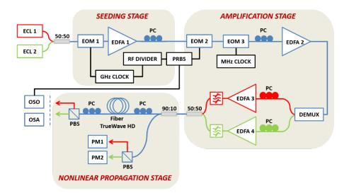
Figure 4 | Experimental setup, red and green lines depict the two wavelength-division-multiplexed and orthogonally polarized pumps. ECL: external-cavity diode laser; 50/50 & 90:10: fiber couplers; EOM: (intensity or phase) electro-optic modulator; EDFA: Erbium doped fiber amplifier; PRBS: pseudo-random binary sequence generator; PC: polarization controller; PM: power-meter; OSO: optical sampling oscilloscope; OSA: optical spectrum analyzer.
