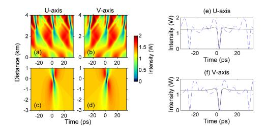
Figure 5 | Contour plots of optical intensity in orthogonal polarization modes. **a**,**b**, numerical solutions showing the generation a periodic train of optical black holes from an initially temporally modulated background (note that distance of light hole center is arbitrarily shifted at origin). **c**,**d**, Exact solution of an isolated black hole. **e**,**f**, Comparison of temporal intensity profiles obtained in the previous panels at black hole centers.
