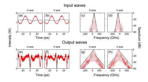
Figure 6 | Experimental observation of the optical ORRW. **a,b**, Temporal profiles of power in the U and V polarization modes at the fiber input (red solid traces). **c,d**, Power spectra at the fiber input. **e,f**, Output intensities after 3 km of optical fiber. **g,h**, Power spectra at the fiber output. Solid black lines represent the analytical black hole solution.
