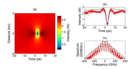
Figure 7 | **a**, Contour plot of the total intensity of the ODRW solution, note that distance of black hole center is arbitrarily shifted at origin. **b**,**c**, Comparison between analytical (black lines) and experimental results (red lines) at the optical ODRW center in both time and spectral domains, respectively.
