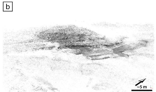
Sparse point cloud 530 cameras (NavCam) 565 271 points
