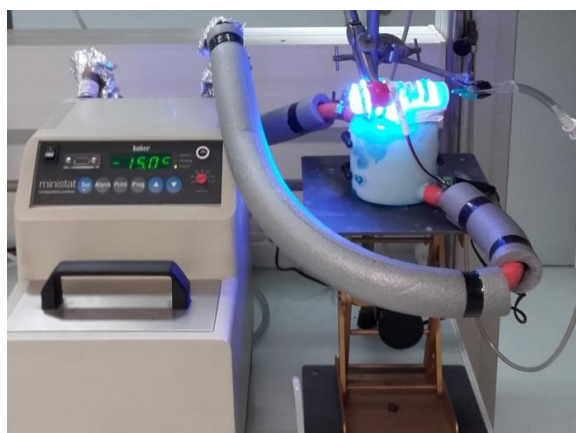
Figure S1. Experimental setup showing a) the cooling unit, the reactor wrapped in the LED strip and b) the reactor with the argon inlet and the needle for introduction of the solution.
