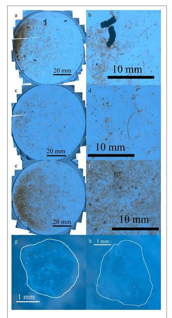
**FIGURE 6** | Representative images of particles collected in acrylamide gel sediment traps showing all particles **(a,c,e)**, or magnified images of a subset of the particles **(b,d,f)**. Images are from P1706-1, 150 m **(a,b)**; P1706-3, 150 m **(c,d)**; P1706-4, 50 m **(e,f)**. **(g,h)** Show representative images of the porous marine snow aggregates that were seen floating on top of the gels.
