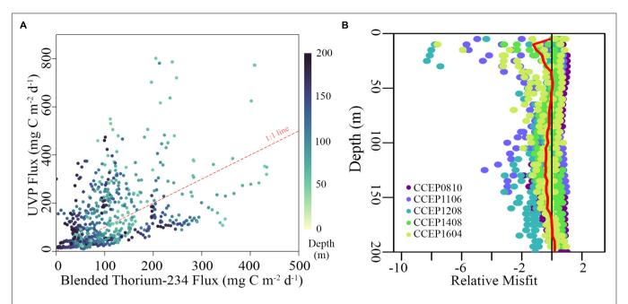
**FIGURE 9 | (A)** Blended  $^{234}$ Th-sediment trap flux estimates from 50 to 200 m compared to estimates predicted by the UVP algorithm using the optimized A and B values of 15.4 and 1.05 respectively. Points are colored by depth and the red dashed line is 1:1. **(B)** Misfit between the UVP flux estimate and the blended  $^{234}$ Th-method [i.e.,  $(F_{UVP} - F_{Th})$ ] plotted against depth, with a red line denoting the mean relative misfit (equivalent to AE) across all cruises.
