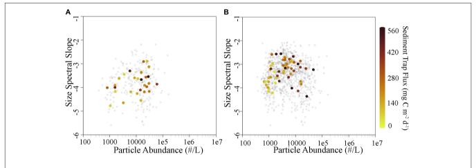
FIGURE 4 | (A) Size spectral slope of particles for the mixed layer (0-20 m) colored by sediment trap flux at 100 m. (B) Same as (A) at each sediment trap deployment depth colored by the flux at that corresponding depth. Gray points are individual cast measurements, while colored points are cycle averages.
