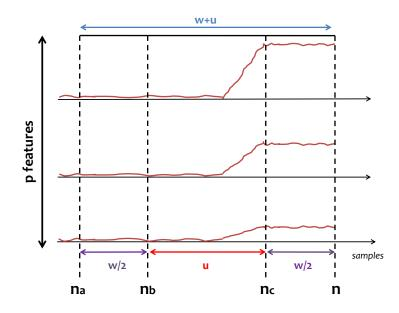
Figure 3: Sliding "Window with Margins" method adjusted to the multivariate case (p=3 features).
