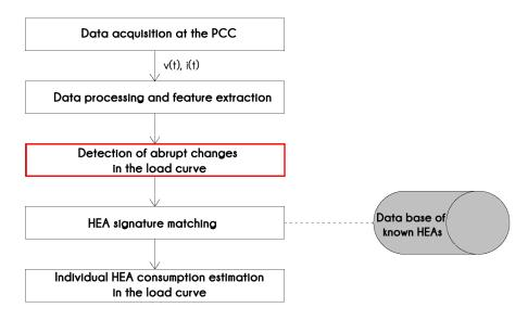
Figure 1: Block diagram of the event-based NILM approaches.
