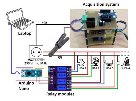
Figure 8: Electrical assembly and instrumentation of four HEAs using our acquisition system [25]
