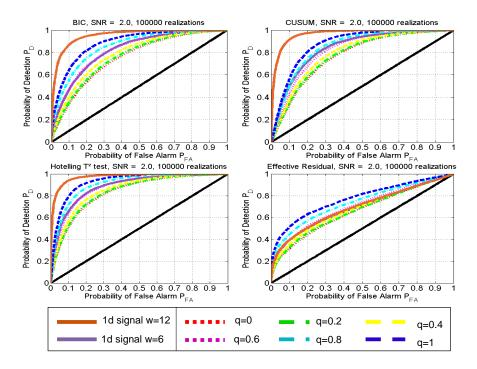
Figure 5: ROC curves of the four studied detectors considering one- and multi-dimensional cases with different step heights in the second dimension.
