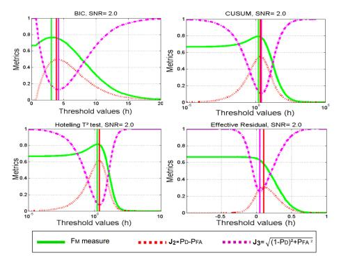
Figure 7: Three metrics values,  $F_M$  (Eq. 28),  $J_2$  (Eq. 29) and  $J_3$  (Eq. 31) against threshold values h of each detector for a fixed SNR value.
