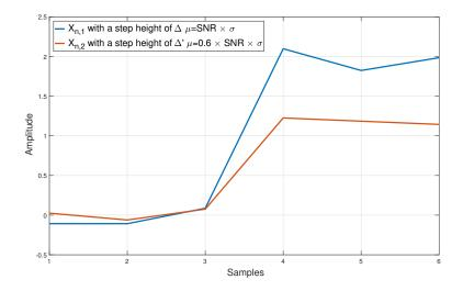
Figure 4: Example of a realization obtained in the Monte Carlo experiment with SNR=20,  $\sigma = 0.1$  and  $\Delta \mu' = 0.6 \times \Delta \mu$ .
