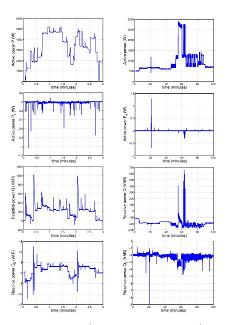
Figure 2: Active power signal, its 4<sup>th</sup> harmonic, reactive power signal and its 5<sup>th</sup> harmonic related to the same scenario of HEAs switched on and off (using our own acquisition system at the left and an extract from the phase B of BLUED dataset at the right).
