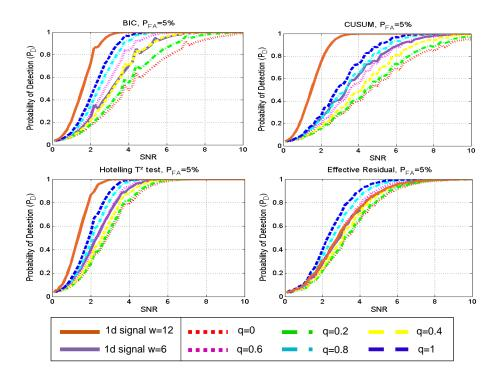
Figure 6: Probability of Detection  $P_D$  (Eq. 26) of the four studied detectors for a varying SNR value with a Probability of False Alarm  $P_{FA} = 5\%$  (Eq. 27) for the one- and two-dimensional cases.
