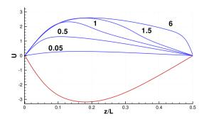
**Fig. 12.** Axial profiles of U at r = 0 (in blue) for corresponding times expressed in  $10^{-3}$  s and at  $r = R - 3\delta_v$  (in red) in the lid-driven cavity for  $U_w$  from  $N_2$ . (For interpretation of the references to color in this figure legend, the reader is referred to the web version of this article.)
