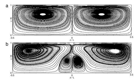
Fig. 1. Streamlines of streaming velocity fields without (a) and with (b) the extra contra-rotating cell (results of numerical simulations  $N_1$  and  $N_2$ ).
