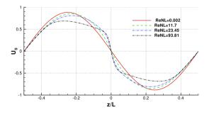
**Fig. 14.** AMS results for streaming velocity scaled by  $3 \times U_{\text{max}}^2/(8c_0)$  along the axis,  $R/\delta_v = 40$ .
