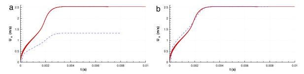
**Fig. 10.** (a) Time evolution (—) of U(z = L/4, r = 0) in lid-driven cavity for  $U_w$  from  $N_2$ , and (——) of  $U_s$  at  $O_c$  from Fig. 6. (b) Same with both curves normalized to reach the same steady-state value. (For interpretation of the references to color in this figure legend, the reader is referred to the web version of this article.)
