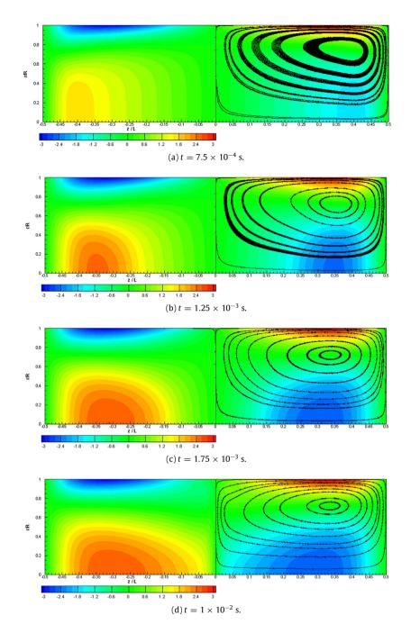
**Fig. 11.** Contours of the axial velocity (with color code) at different times during the transient evolution in the lid-driven cavity for  $U_w$  from  $N_2$ . Streamlines are superimposed on the right half plane section. (For interpretation of the references to color in this figure legend, the reader is referred to the web version of this article.)
