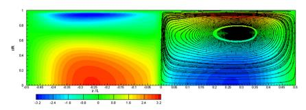
**Fig. 16.** AMS results,  $R/\delta_v = 50$ . Isolines of the axial streaming velocity colored by its value and the streamlines of the streaming flow. (For interpretation of the references to color in this figure legend, the reader is referred to the web version of this article.)
