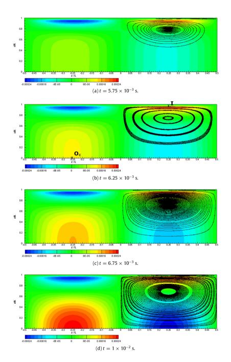
**Fig. 3.** Contours of the axial streaming velocity (with color codes in m/s) at different times during the transient evolution of  $N_1$ . Streamlines are superimposed on the right half plane section (real aspect ratio height/length=0.09). (For interpretation of the references to color in this figure legend, the reader is referred to the web version of this article.)
