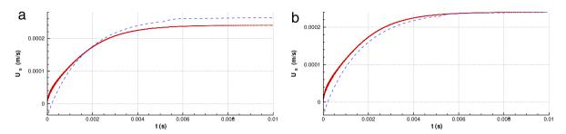
**Fig. 9.** (a) Time evolution ( —) of U(z = L/4, r = 0) in lid-driven cavity for  $U_w$  from  $N_1$ , and ( — —) of  $U_s$  at  $O_c$  from Fig. 4. (b) Same with both curves normalized to reach the same steady-state value. (For interpretation of the references to color in this figure legend, the reader is referred to the web version of this article.)
