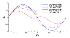
**Fig. 15.** Dimensionless streaming velocity along the axis. Comparison of DNS (solid lines), AMS (dashed lines) and Lid-Driven Cavity, LDC (dashed-dotted lines) results,  $R/\delta_v = 50$ , for slow-streaming (in blue) and fast-streaming (in red). (For interpretation of the references to color in this figure legend, the reader is referred to the web version of this article.)
