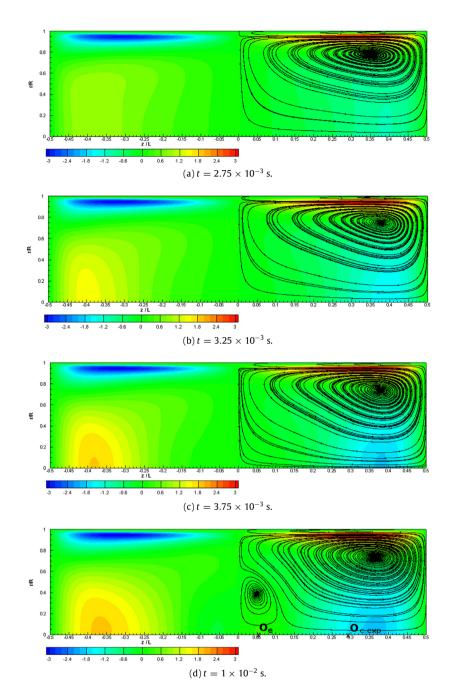
**Fig. 5.** Contours of the axial streaming velocity (with color code) at different times during the transient evolution of  $N_2$ . Streamlines are superimposed on the right half plane section (real aspect ratio height/length = 0.09). (For interpretation of the references to color in this figure legend, the reader is referred to the web version of this article.)
