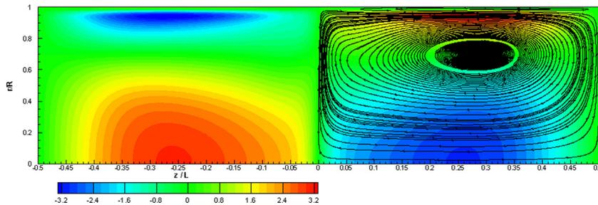
**Fig. 16.** AMS results,  $R/\delta_v = 50$ . Isolines of the axial streaming velocity colored by its value and the streamlines of the streaming flow. (For interpretation of the references to color in this figure legend, the reader is referred to the web version of this article.)
