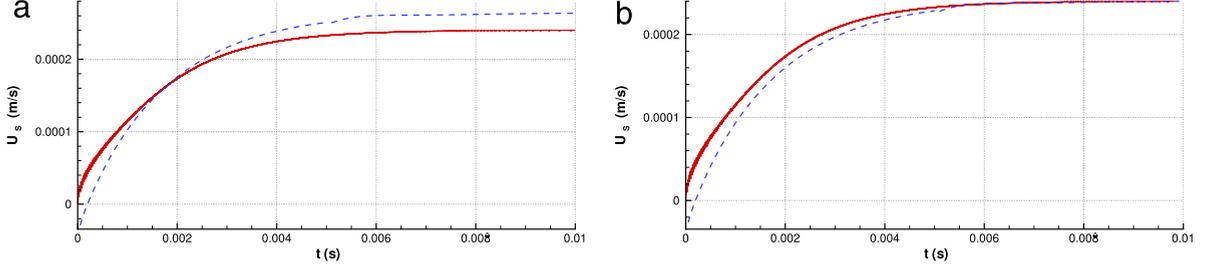
**Fig. 9.** (a) Time evolution (—) of  $U(z = L/4, r = 0)$  in lid-driven cavity for  $U_w$  from  $N_1$ , and (---) of  $U_s$  at  $O_c$  from Fig. 4. (b) Same with both curves normalized to reach the same steady-state value. (For interpretation of the references to color in this figure legend, the reader is referred to the web version of this article.)
