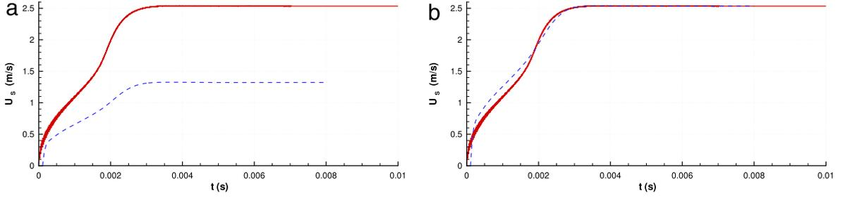
**Fig. 10.** (a) Time evolution (—) of  $U$  ( $z = L/4, r = 0$ ) in lid-driven cavity for  $U_w$  from  $N_2$ , and (---) of  $U_s$  at  $O_c$  from Fig. 6. (b) Same with both curves normalized to reach the same steady-state value. (For interpretation of the references to color in this figure legend, the reader is referred to the web version of this article.)
