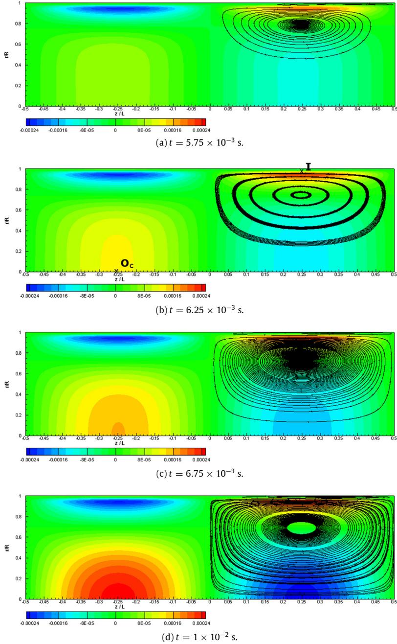
**Fig. 3.** Contours of the axial streaming velocity (with color codes in m/s) at different times during the transient evolution of  $N_1$ . Streamlines are superimposed on the right half plane section (real aspect ratio height/length=0.09). (For interpretation of the references to color in this figure legend, the reader is referred to the web version of this article.)
