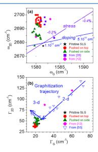
**Figure 2.** (a) Doping and strain characterization with a  $\omega_{2D}$  vs  $\omega_{G}$  plot. Data from Bayle et al. <sup>28</sup> have been  $\lambda_{L}$ -corrected using a 2D band dispersion of 100 cm<sup>-1</sup>/eV. Straight lines correspond to the behavior under doping (blue) or strain (violet). <sup>35–37</sup> (b) Structural characterization with a  $\Gamma_{2D}$  vs  $\Gamma_{G}$  plot.
