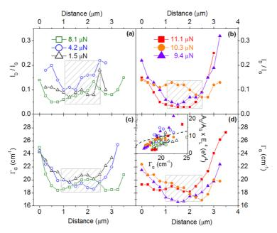
Figure 3. Raman profiles of top pushed graphene zones. (a)  $I_{\rm D}/I_{\rm G}$  profiles for tip forces of 1.5, 4.2, and 8.1 μN. (b)  $I_{\rm D}/I_{\rm G}$  profile for tip forces of 9.4, 10.3, and 11.1 μN. (c,d) Same as (a) and (b) for  $\Gamma_{\rm G}$  profiles. Gray boxes emphasize the zone centers. The inset in Figure 3d represents  $A_{\rm D}/A_{\rm G}$  ×  $E_{\rm L}^4$  as a function of  $\Gamma_{\rm G}$ . The dotted line is from ref 39, with  $L_{\rm D}$  = 500 nm (see text).
