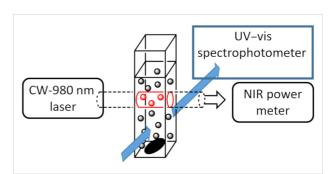
**Figure 2:** UCNPs (black dots) are irradiated inside the cylindrical CW 976 nm laser beam. Absorbed laser power is recorded with a powermeter. The UV–vis spectrophotometer axis is perpendicular to the laser beam.
