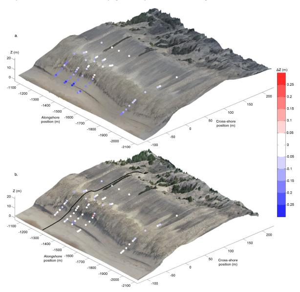
**Figure 4.** Elevation relative error (colored circles) between the DSM, generated using 10 GCPs, and the DGPS ground survey superimposed onto the 3D textured DSM for (a) DP2 and (b) DP4P. The DSM in (a,b) were generated with DP2 and DP4P images, respectively. The black line shows the cross-shore profile presented in Figure 5.
