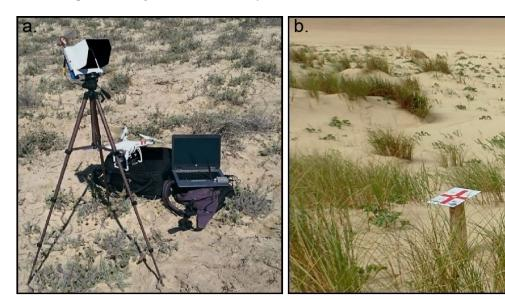
**Figure 2.** The dune survey system composed of (a) light and low-cost UAV hardware, computer ground station, video receiver, and (b) permanent GCPs spaced every 250 m and approximately 50–100 m in the alongshore and cross-shore directions, respectively.
