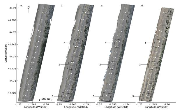
**Figure 6.** Orthophotos of the entire 4-km study area of Truc Vert beach on (a) 9 October 2017, (b) 19 December 2017, (c) 23 January 2018 and (d) 13 March 2018. The positions of the 36 permanent GCPs implemented in 250-m spaced pairs along the entire 4-km dune system used for the DSM generation are indicated by white dots and the black squares show the areas zoomed onto in Figure 7.
