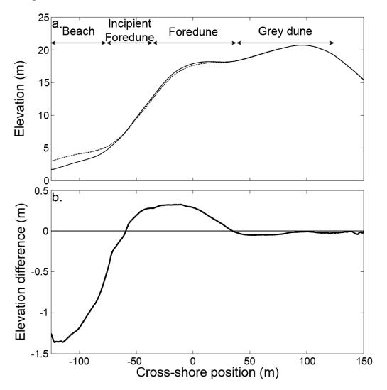
**Figure 8.** (a) 4-km alongshore-averaged beach-dune profile at Truc Vert on 9 October 2017 obtained with DP2 (dotted black line) and on 13 March 2018 obtained with DP4P (black line) with (b) corresponding elevation change between 9 October 2017 (survey performed with DP2) and 13 March 2018 (survey performed with DP4P).
