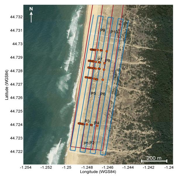
**Figure 3.** Zoom onto the 1-km southern end of the 4-km field size. This 1-km section corresponds to the location of the validation experiment delimited by the dotted white box. P1-P10 indicate the location of the permanent GCPs, the alongshore red lines and blue lines represent DP2 and DP4P flight trajectories, respectively, and the orange dots show the DGPS survey points used for the validation experiment.
