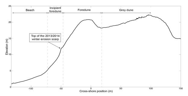
**Figure 5.** Cross-shore profile of the beach-dune system at Truc Vert showing the different morphological compartments with indication of the location of the 2013/2014 erosion scarp mark.
