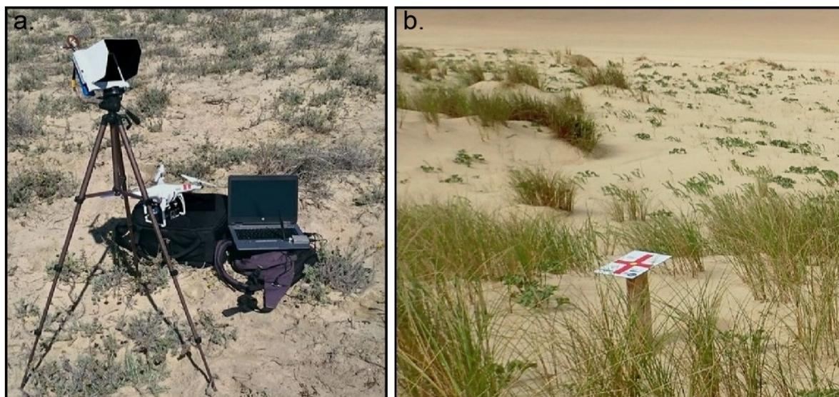
**Figure 2.** The dune survey system composed of (a) light and low-cost UAV hardware, computer ground station, video receiver, and (b) permanent GCPs spaced every 250 m and approximately 50–100 m in the alongshore and cross-shore directions, respectively.
