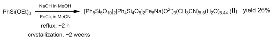
**Figure 2.** General scheme for the synthesis of **II**.
