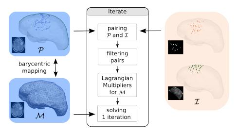
Figure 4: iterative registration process. Pairings between pre- and intraoperative datasets  $\mathcal{P}$  and  $\mathcal{I}$  are computed, then filtered. This defines the directions of the Lagrangian Multipliers constraints, stored in matrix  $\mathbf{H}$ , applied to the biomechanical model  $\mathcal{M}$  so that it deforms towards  $\mathcal{I}$ .
