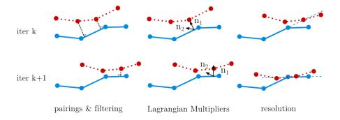
Figure 5: sliding constraints
