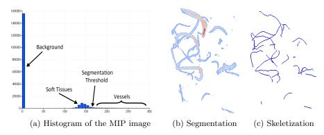
Figure 2: Histogram of the MIP image, segmentation and mesh generation of the vessel tree.
