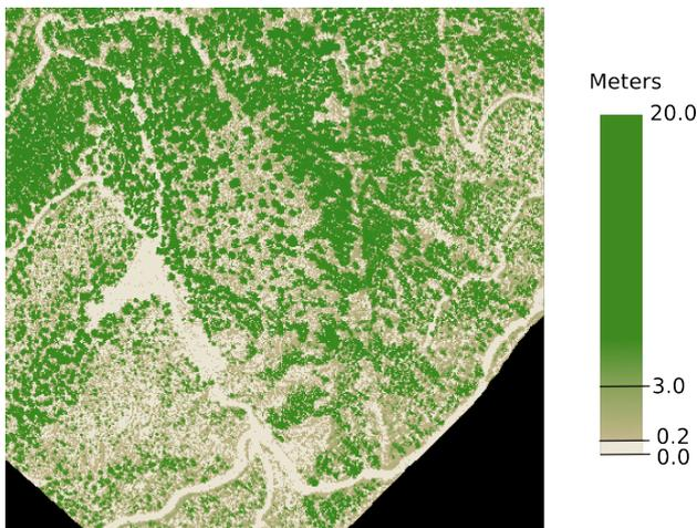
Figure 3: nDSM image generated from the last pulses of the lidar point cloud.
