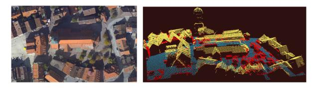
Figure 5: Classification results in a dense urban area (Biberach city). **Left**: orthoimage of the region of interest. **Right**: classified point cloud (yellow: buildings, red: vegetation, blue: artificial ground and green: natural ground).
