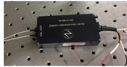
Figure 5. Left: Optical path inside the delay line. The input beam reflects on a movable mirror and is then re-injected in the output fiber. Right: Picture of a delay line.
