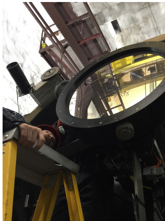
Figure 1-1: Rotatable spider structure of the UH-88 inch telescope that allows interchanging one of the (current) passive secondary mirrors by the Adaptive Secondary Mirror system that is currently under design.
