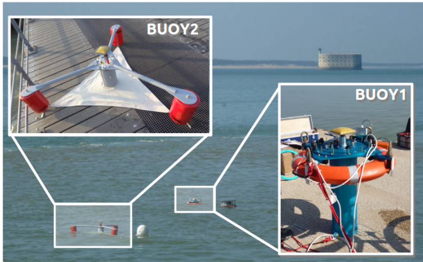
FIG. 2. The two GNSS buoys: BUOY1 and BUOY2.
