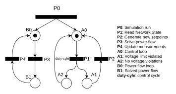
Fig. 4. Power flow analysis and production control, running in parallel
