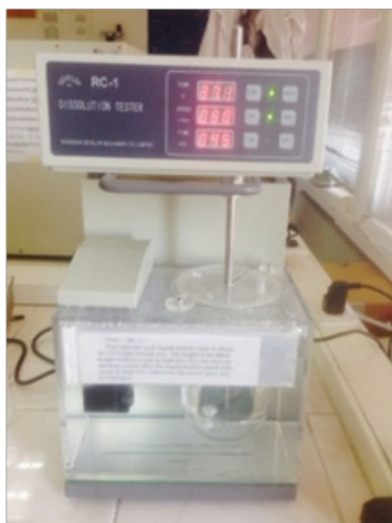
Figure 2 Develop (RC-1) Dissolution Tester machine, PAN/SBA-15 in PBS solution under stirring.
