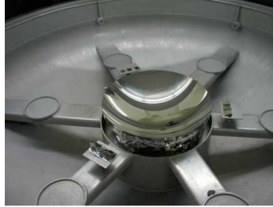
Fig. 3 Secondary Reflector: reflective coating
