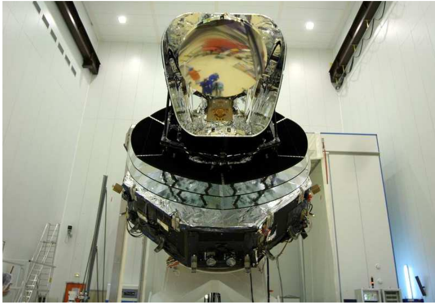
Fig. 1 the Planck Satellite, on mounting fixture, during the ground tests. The telescope (primary mirror) and the thermal baffle are visible in the foreground
