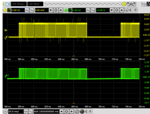
Figure 12: Emitted and received baseband waveforms
