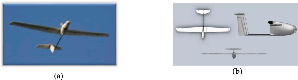
Figure 1. OVLI-TA UAV (a,b) based on the commercial airborne model Techpod, manufactured by HobbyUAV.
