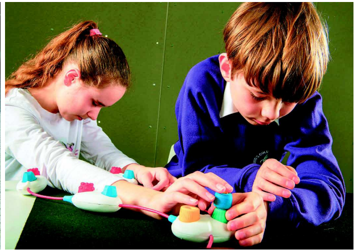
Two children with visual impairments collaborating using Torino, a socially inclusive physical programming language for teaching basic programming constructs and computational thinking skills.
