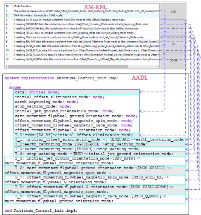
Fig. 14. Traceability link of the attitude control subsystem.
