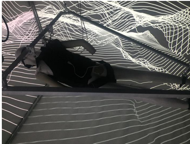
Fig. 8. A camera and the binaural microphones are attached on the head of mannequin.
