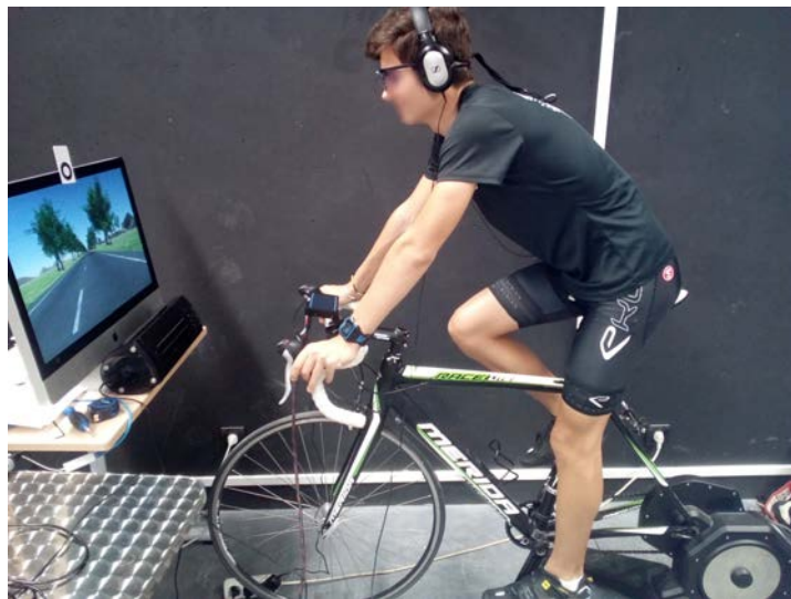
Figure 1: Experimental setup: 27" screen displaying a virtual road, 5" screen on the handlebars reporting visual feedback, bike Merida, Home-Trainer Tacx. The cyclist is wearing headphones during the Auditive condition, and is wearing Tobii glasses during the whole experiment.
