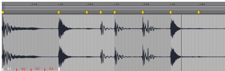
Fig. 2. First bar of a drum break from Aerosmith - Walk This Way to illustrate what can go wrong with fixed length segmentation. Between the first 4 segments, only S1 contains an onset — is an event —, although the drum lasts at least 3 more steps. We associate the event with its length. In this case the length is 4 segments because the next event is located in S5. So, the sample 1 includes the segments S1, S2, S3, S4.
