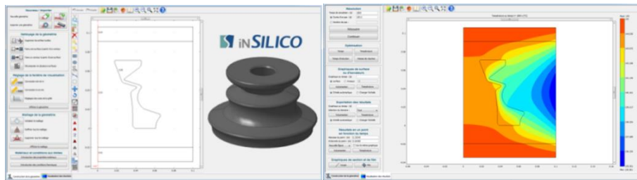
Fig. 5. Geometry design (left) and temperature fields obtained (right) with the multi-physical model
