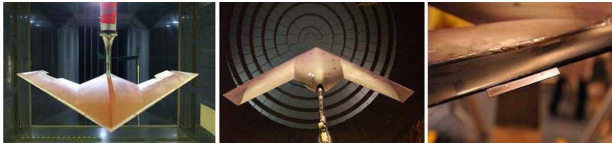
Fig. 2 SACCON model belly-mounted upside down in DNW-NWB low-speed wind tunnel (left), model in ONERA-L1 (middle), and details of the leading-edge slat (right).
