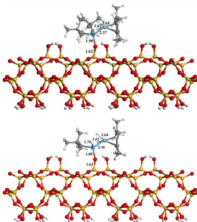
**Figure 7.** DFT optimized structures of the silica-supported complexes **5** (top) and **6** (bottom – model 6a; model 6b in SI). Selected bond distances are given in Å. Ta is represented in blue, Ir in green, Si in yellow, O in red, C in grey and H in white.
