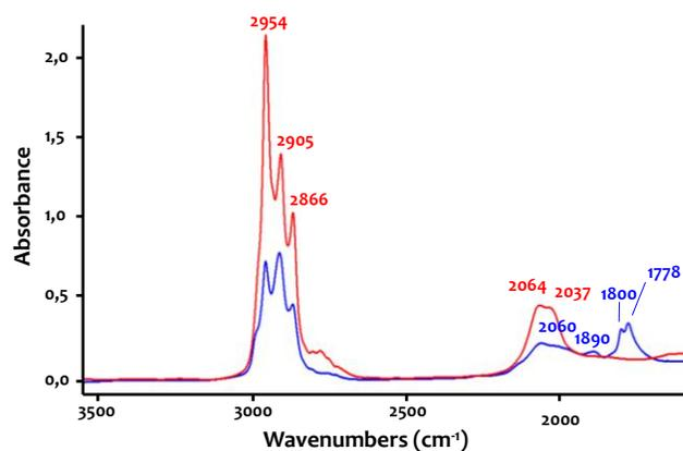
**Figure 5.** Infrared spectra of **5** (red line) and **6** (blue line) recorded in transmission on pelleted materials under argon. The SBA-15<sub>700</sub> signal has been subtracted to remove contribution from the support.
