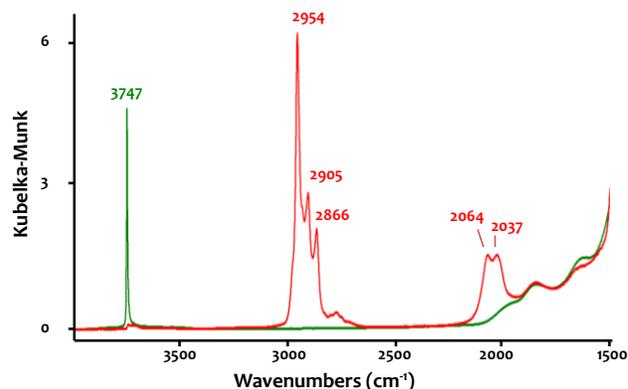
**Figure 2.** Diffuse reflection infrared Fourier transform spectra of SBA-15<sub>700</sub> (green line) and compound **5** (red line) recorded on powder materials under argon.
