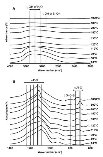
Figure 7: FTIR spectra of the sample measured at various temperatures between 4000-2000 cm<sup>-1</sup> (A) and 1400-600 cm<sup>-1</sup> (B) with the main positions of (-) AlPO<sub>4</sub> hydrated, (-) AlPO<sub>4</sub> berlinite, (--) AlPO<sub>4</sub> tridymite and cristoballite, (..)  $\delta$  Si-O-Si.
