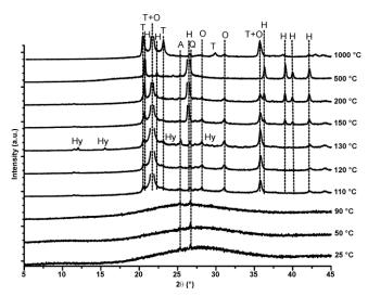
Figure 6: XRD patterns of the sample treated at various temperatures. In this figure are flagged the positions T: trydimite-type  $AlPO_4$  (01-070-4689), O: cristobalite-type  $AlPO_4$  (01-072-1161), H: berlinite  $AlPO_4$  (01-089-4201), Hy: hydrated aluminophosphate such as  $Al(H_2PO_4)_3$  (01-14-0377) and  $Al(H_2PO_4)(HPO_4)H_2O$  (00-76-376), A: anatase (01-071-1166) and Q: quartz (00-046-1045).
