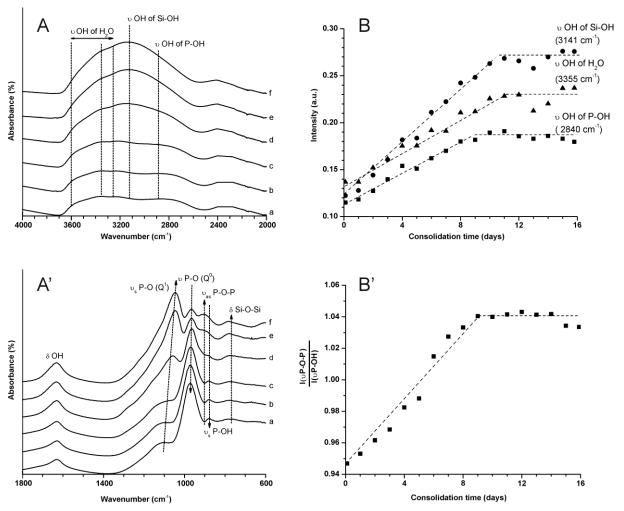
Figure 2: FTIR spectra of the sample measured between (A) 4000-2000 cm<sup>-1</sup> and (A') 1800-600 cm<sup>-1</sup> at 0 (a), 1(b), 3(c), 7(d), 14(e) and 20 days (f) of consolidation. (B) evolution of the intensity of v M-OH (M=H, Si and P). (B') evolution of  $\frac{I(v_{as} P - 0 - P \text{ at } 902 \text{ cm}^{-1})}{I(v_s P - 0 H \text{ at } 880 \text{ cm}^{-1})}$  as a function of the consolidation time.
