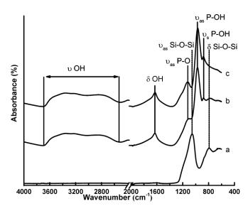
Figure 1: FTIR spectra of the metakaolin (a), the initial reactive mixture (b) and the diluted phosphoric acid (c).
