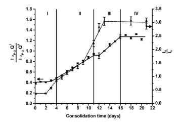
Figure 8: evolutions of the  $\frac{I v P - O Q^1 (1045 cm^{-1})}{I v P - O Q^0 (970 cm^{-1})}$  ratio from FTIR spectra (black squares) and of the  $\frac{I_G}{I_S}$  ratio from XRD patterns (open circles) as a function of the consolidation time.
