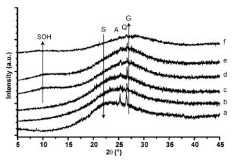
Figure 3: diffractograms of the metakaolin (a), of the binder at days 1(b), 2(c), 8(d) and 9(e) of consolidation and of the consolidated geopolymer (f). In this figure are flagged the positions of anatase (A: 01-071-1166), quartz (Q: 00-046-1045) and of the contributions assigned to hydrated silica (SOH), silica (S) and geopolymer (G) networks.
