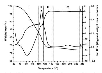
Figure 5: thermal analysis of the geopolymer ((a) heat flow, (b) weight loss and (c) weight loss derivative) shown between 20 and 240  $^{\circ}$ C.
