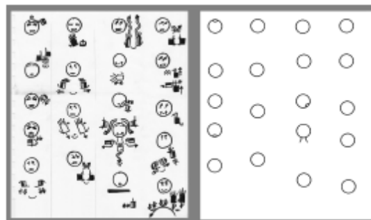
Fig. 5. Screenshot taken from SW-OGR during the development phase (ongoing). The image shows a handwritten text (courtesy of ISTC-CNR) and the result of the detection routine for the head symbols.
