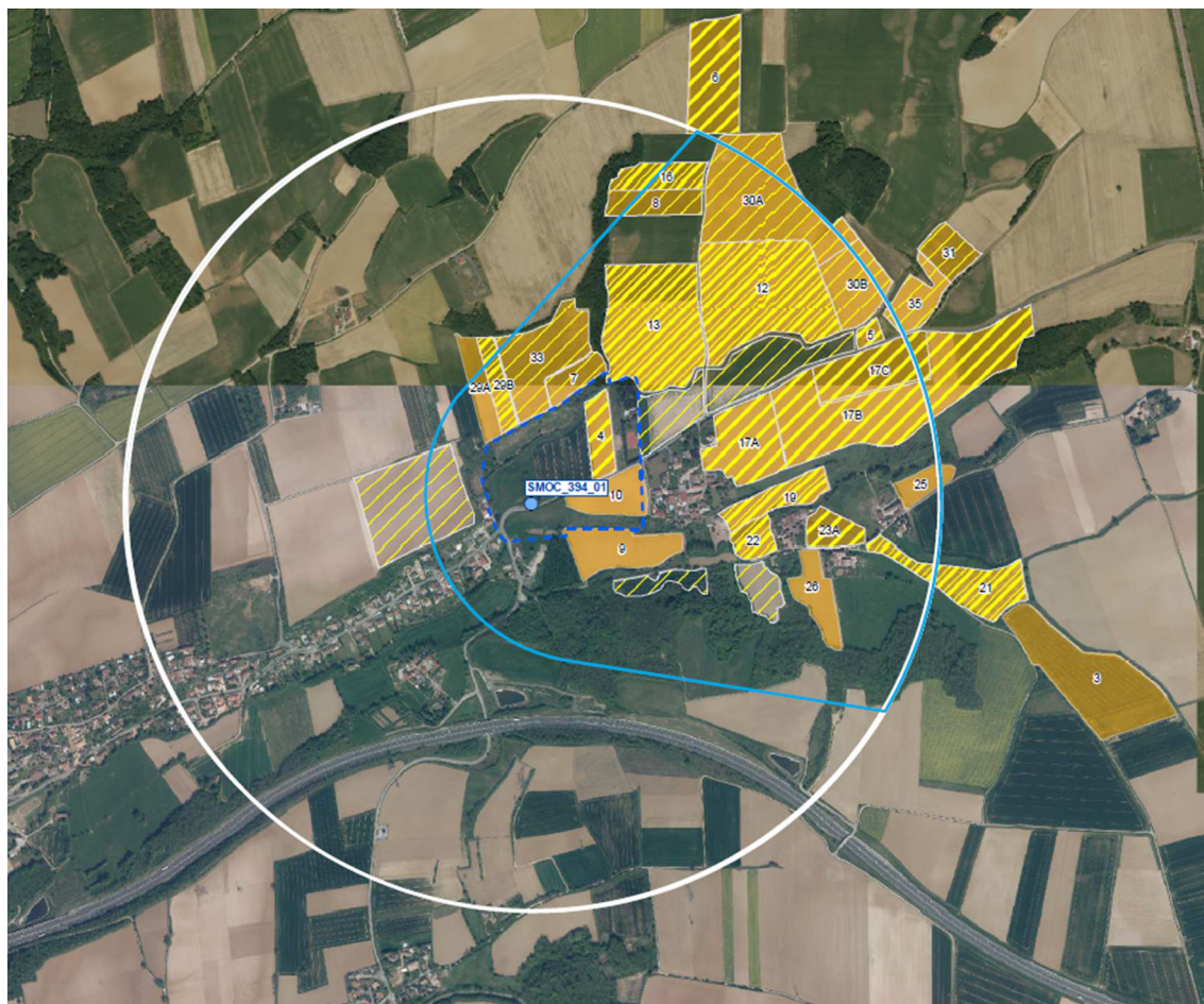
Fig. 9 Investigation example of the recharge/catchment area in a well to collect the use history of an active substance, agronomic practices, soil information, and aquifer characteristics. The fields in yellow indicate cultivation of the targeted crop, yellow and thin hatching indicate cultivation of targeted crop and use of targeted compound the
