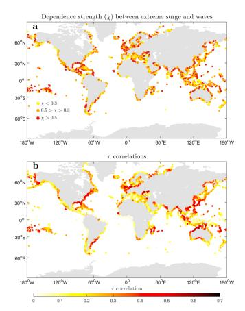
Figure 1. (a) Dependence strength between extreme storm surges (events exceeding the 99th percentile) and concurrent waves, as measured by  $\chi$ . Blank coastline segments indicate that there is not asymptotic dependence between extremes (limiting value of  $\bar{\chi} < 1$ , see text for details). (b) Map of Kendall  $\tau$  correlations between the same extremes storm surges and concurrent waves.
