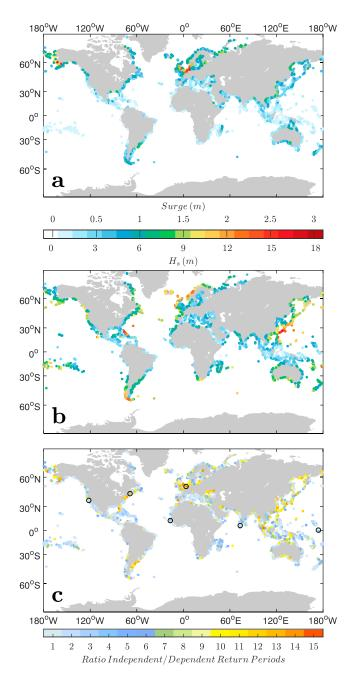
**Figure 2.** The 50-year joint return levels for surges (a) and for  $H_s$  (b) computed for the coastal grid points where there is dependence. (c) Ratio between the joint return period (50-year) and the independent return periods assuming independence, with selected grid points highlighted.
