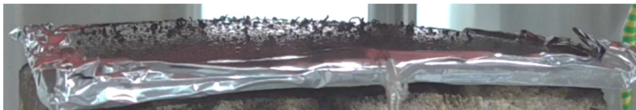
Fig. 3. Charring of the formulation PP-AP760/EG (9:1) before the ignition
