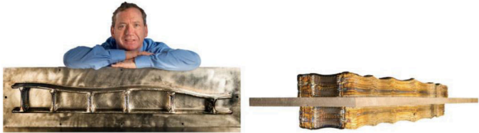
Fig. 45. Ti-6Al-4V wing spars (1.2m long) built back-to-back on a sacrificial build plate for BAE Systems [352]: side view show one wing spar (left) and top view showing both wing spars (right).
