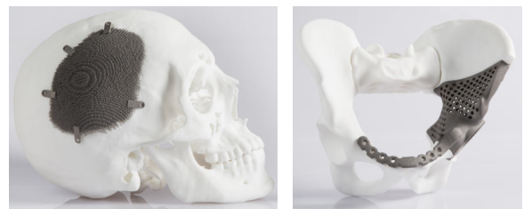
Fig. 18. Titanium implants for the skull (left, [103]) and pelvis (right, [107]) produced using and EOSINT M 280.
