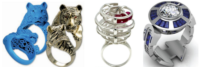
Fig. 9. Jewellery produced with AM: award winning Tiger Ring from OG-Art - pattern printed in wax on a Solidscape machine (via [34]) (left), Kinetic Ring from Vulcan Jewelry (available for purchase) (center, courtesy of Vulcan Jewelry); custom R2D2 inspired ring from Uptown Diamond and Jewelry - pattern printed in wax on a 3D Systems ProJet machine [4] (right).
